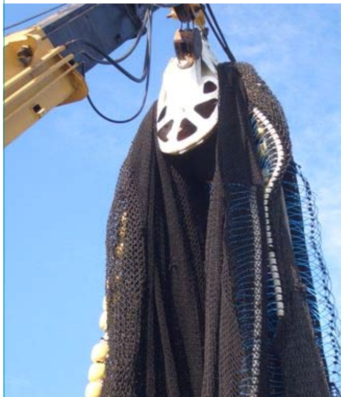
PLATE 3 Flexible sorting grid going through the power block.
