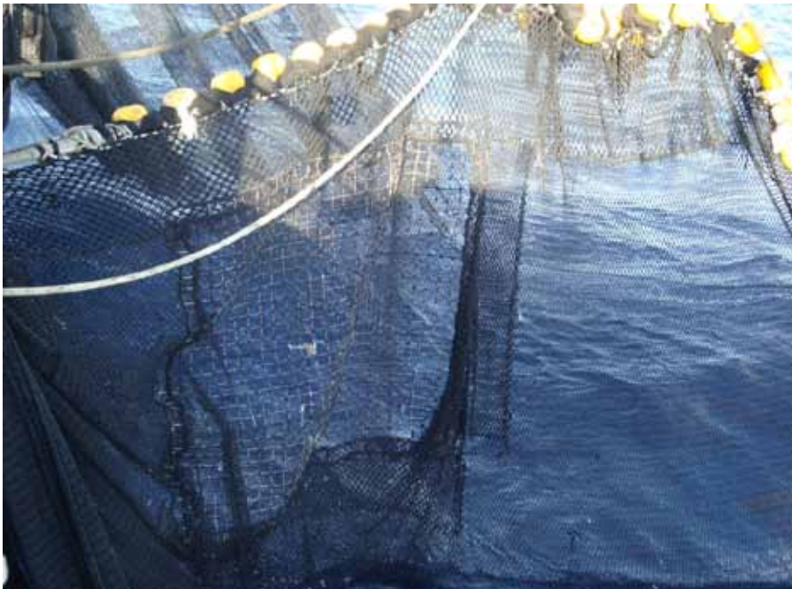
PLATE 7 Villar's sorting grid in the water.
