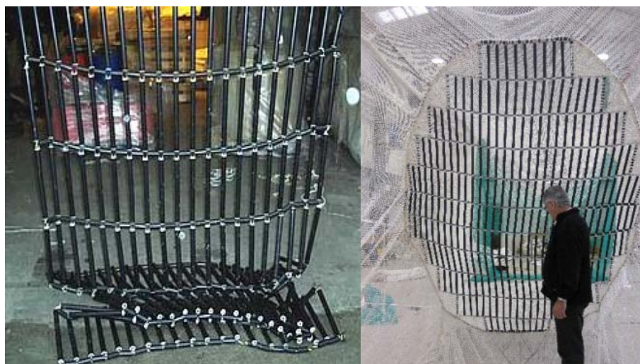
PLATE 8 Zachariassen's grid used in trawls.
