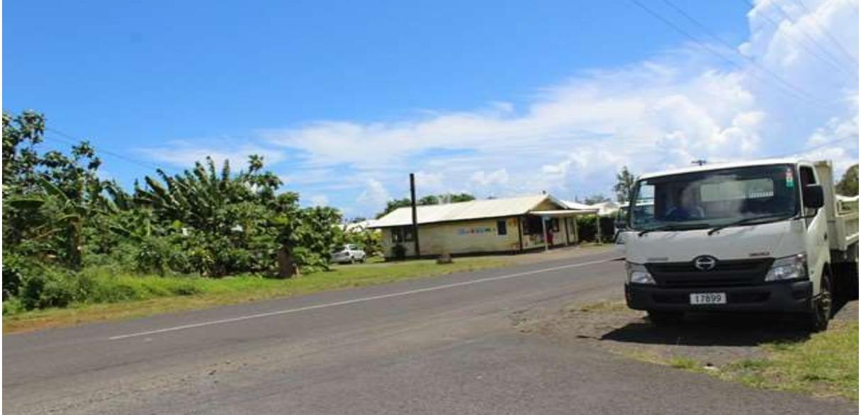
Lotopa village biggest problem is no roadside drainage as shown in the picture making it vulnerable to flooding
