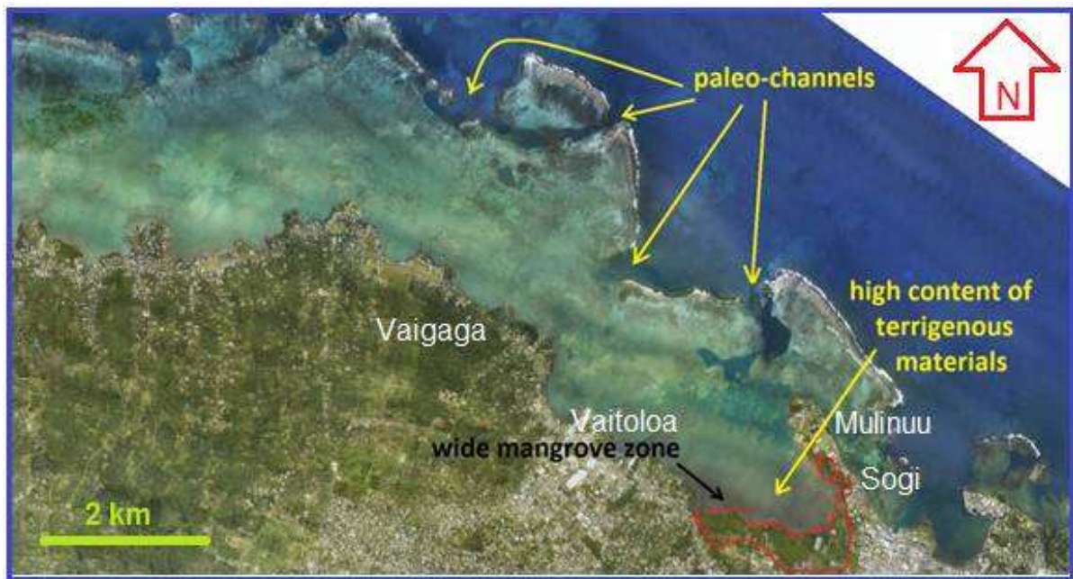
Figure 1 Coastal section between Sogi and Vaiusu with a broad mangrove zone dominated by terrigenous materials. Reef channel networks to the northwest of Mulinuu responsible in transporting great volume of sand in deep water
