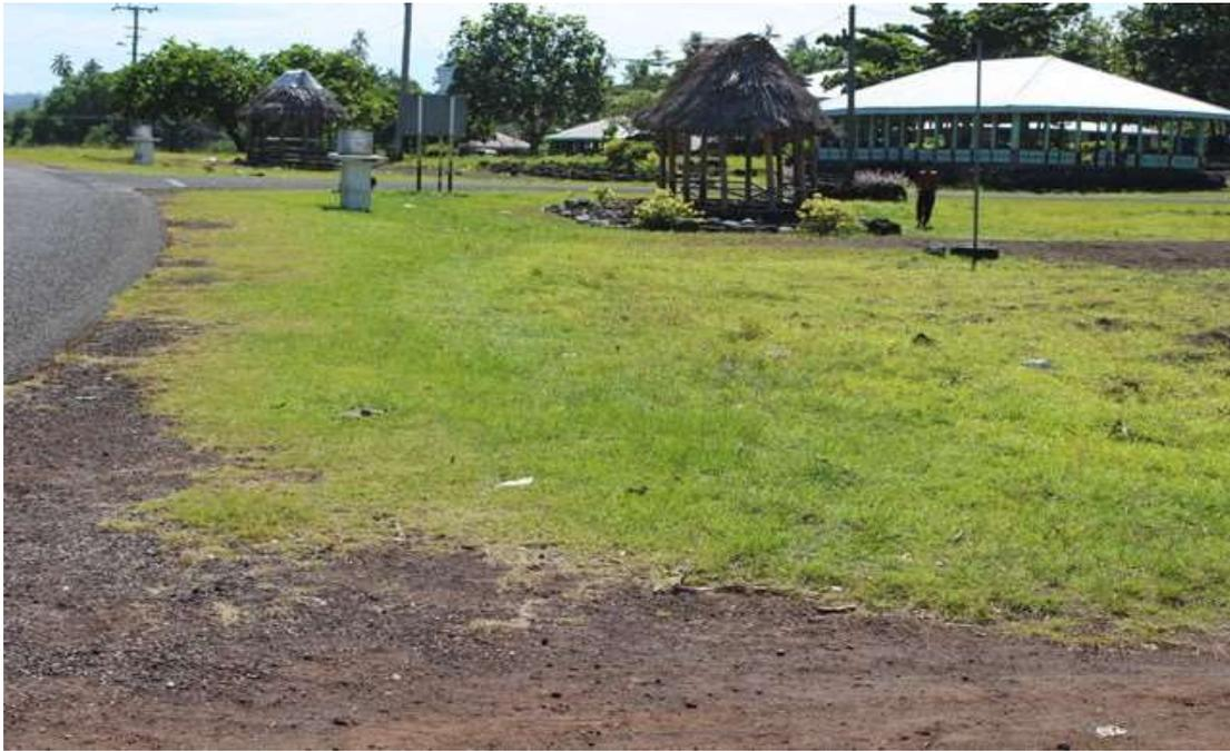
Sasina Village main road - has no road side drainage and prone to flooding.
