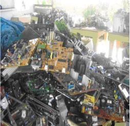
CRTs from computers monitors and televisions have been disassembled and ready for packing. The valuable components from printed circuit boards, and marketable chips for reuse, as well as substantial quantities of copper, gold, silver and palladium can be recovered in New Zealand at an appropriate recycling facilities.
