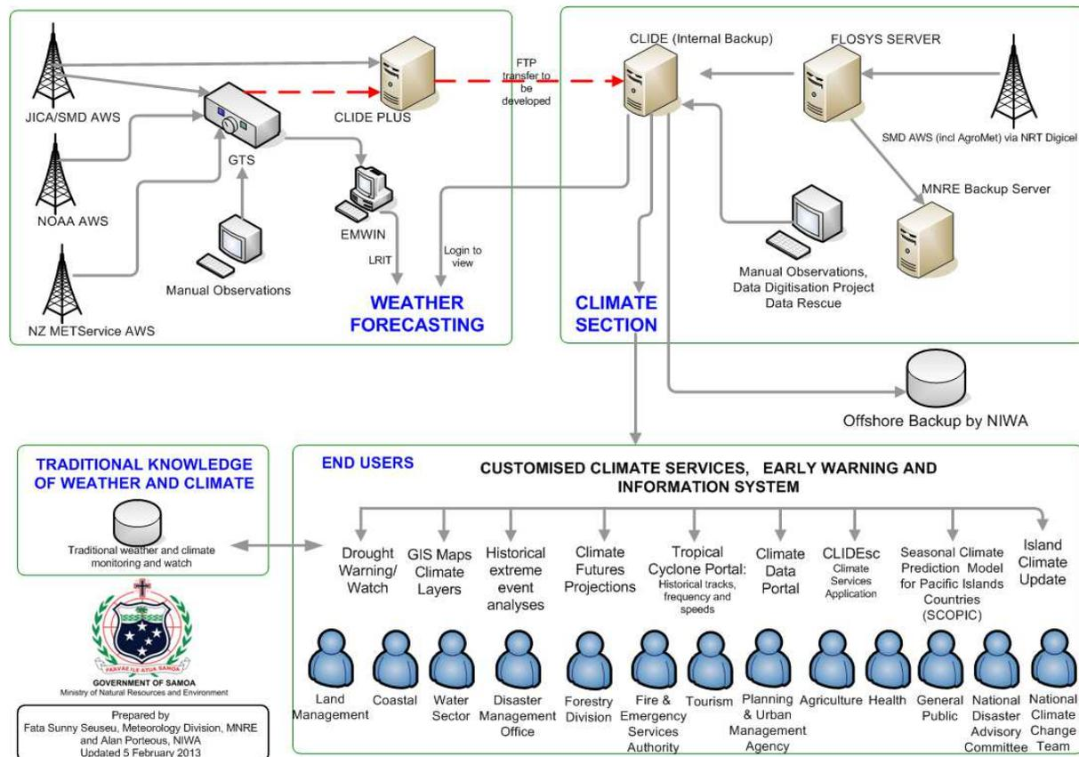
**Figure 3.2: A schematic view of the structure and pathways of data services, weather forecasting and climate services accessed from, or centred at, Samoa Met Division, Apia. The blue ‘end user’ icons indicate the need and scope to build climate services in Samoa. Source: Sunny Seuseu, Samoa Met Division.**
