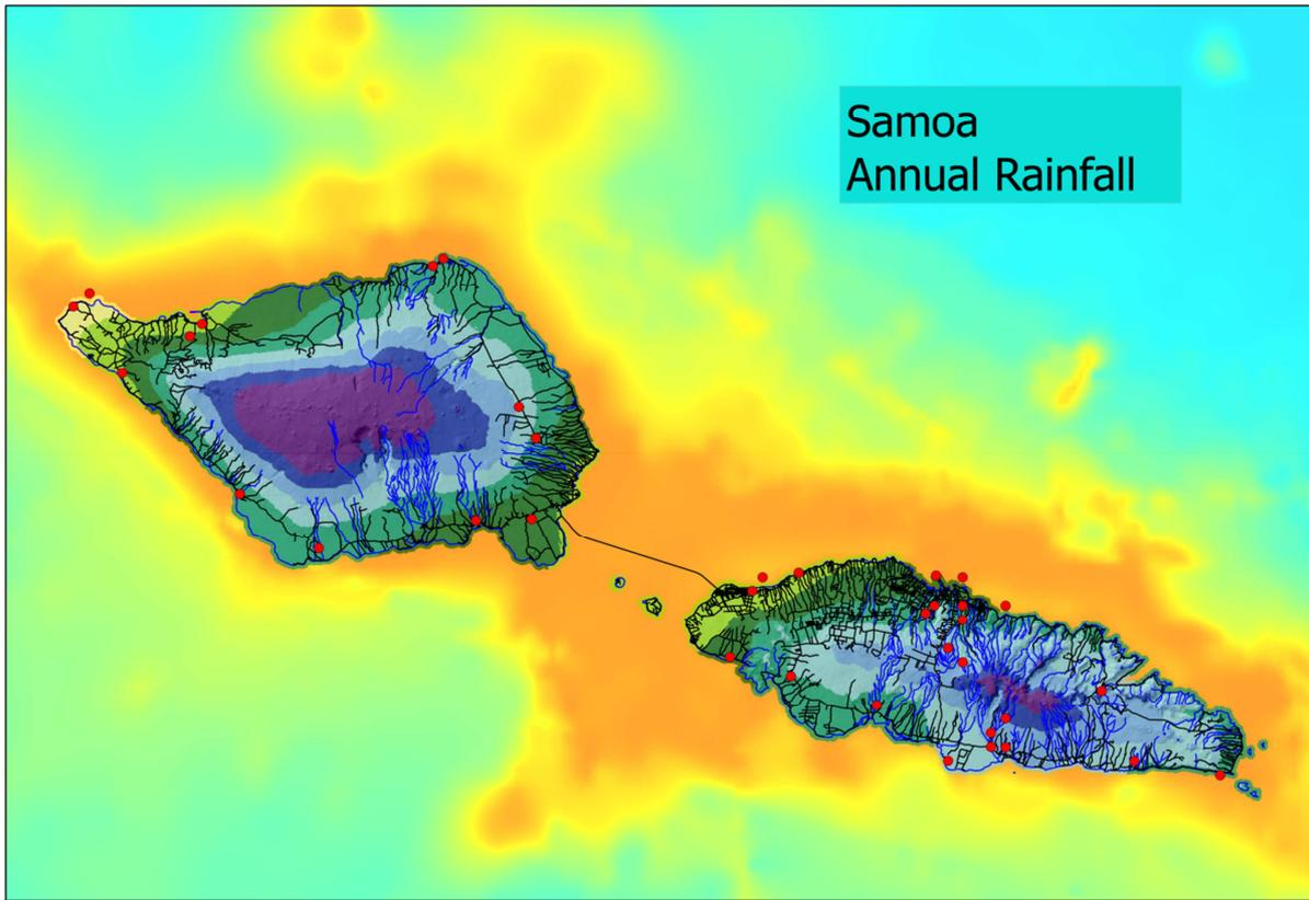
A base map of Samoa produced in Quantum GIS, showing topography, bathymetry, station locations, rivers, roads, coastline and annual rainfall. Climate data surfaces, such as rainfall anomaly maps, produced in Quantum GIS can be exported for use on other GIS platforms. The software is designed for easy importing of geo-referenced data, such as agricultural or health risk data sets.
