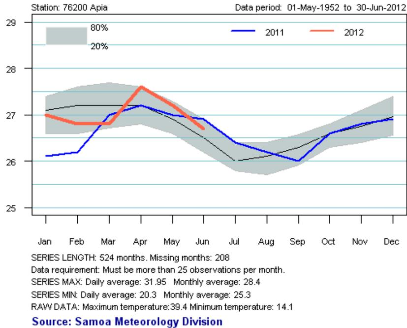
Example CliDEsc product: Monthly average air temperatures at Apia. The grey band shows the 20<sup>th</sup> and 80<sup>th</sup> percentile values, and the black curve is the median.
