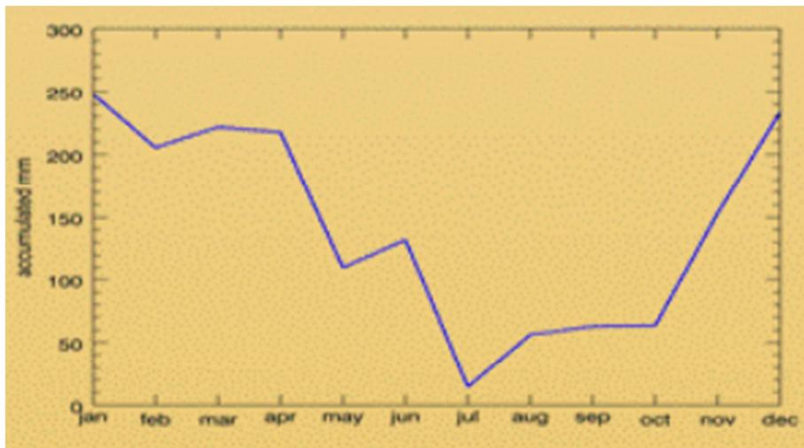
**Precipitation estimates derived from NASA TRMM capturing the 2009 seasonal cycle of rainfall for a satellite grid box within Savaii. A dry season is visible throughout the mid-summer month of July. Interannual comparison of these data would help determine the relative severity of annual dry period rainfall deficits.**
