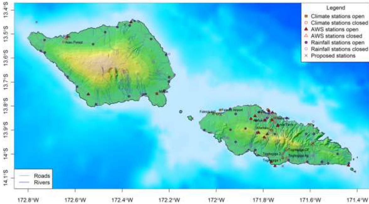
Example CliDEsc product: Location of climate stations in Samoa. The map also shows terrain elevation data, roads, rivers and bathymetry.
